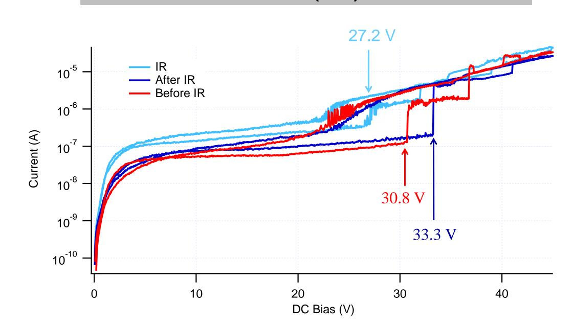
The Near IR radiation excites electron hole pairs in the nanoconstriction so the sample responds to the same biases with a higher current. This effect is washed out with the onset of impact ionization. The log of the current versus DC Bias shows that the IR does affect the voltage at which impact ionization occurs, beyond the error of the stochastic behavior.
